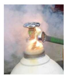
A fire cannot backflash into cylinder since there is no oxidizer inside
