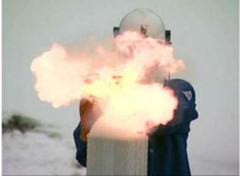
The most likely point for a leak in preparing a silane cylinder for use is when the vaportight outlet cap is removed. So that the operator is not surprised or injured, they must be properly trained and fully clothed in proper PPE. The following are the minimum guidelines that should be followed:
