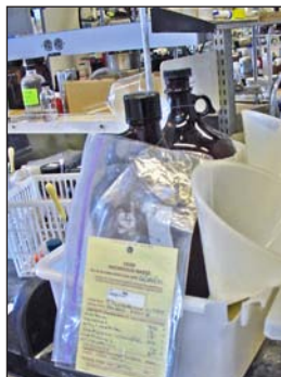
Properly labeled, capped waste in secondary containment.
