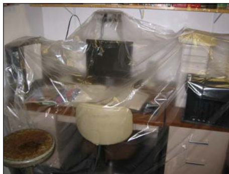
Equipment protected from overhead flooding with plastic sheeting.
